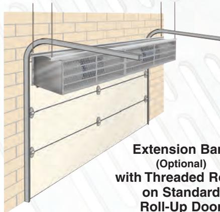
**Extension Bars (Optional) with Threaded Rods\* on Standard Roll-Up Door**
